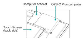
Schematic diagram after the assembly of the OPS-C Plus computer
