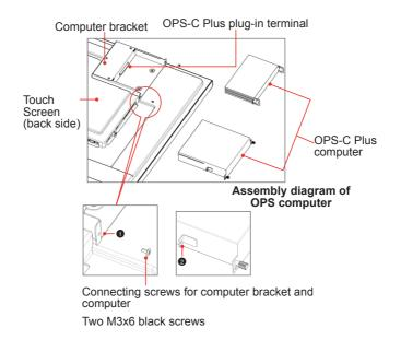
(1) is located at the computer bracket and the connecting screw of computer, which can be matched with (2) .
