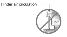
Insufficient ventilation will overheat the device and may cause damage to the device and even fire.
