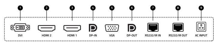
① DVI - ② HDMI2 - ③ HDMI1 - ④ DP-IN - ⑤ VGA - ⑥ DP-OUT - ⑦ RS232(RJ45)/IR IN - ⑧ RS232(RJ45)/IR OUT - ⑨ AC INPUT
